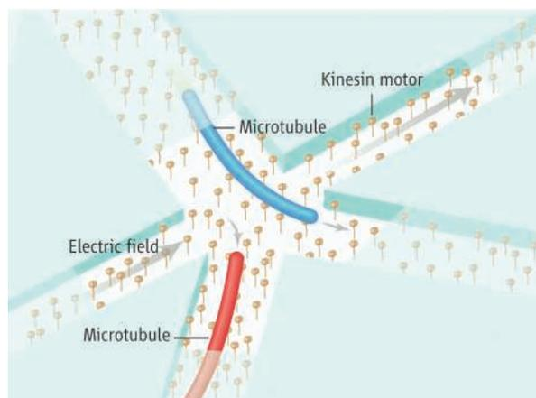
**Nanofluidics with molecular motors.** In van den Heuvel *et al.*'s work (2), an electric field is used to steer the microtubules into one of two arms of a Y junction; the microtubules move perpendicular to the field. The microtubules are transported by kinesin motor proteins.
