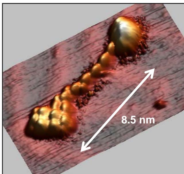
**Figure 4** Monomolecular Co-TPA ‘wire’ linking two cobalt nanodots. The Co island rims are also decorated by molecules. This 1D structure coexists on the surface with regions covered by nanogrids (doses: 0.2 ML Co, 0.2 ML TPA; sample kept at 360 K during TPA deposition; image size  $15 \times 8 \text{ nm}^2$ ,  $V = -700 \text{ mV}$ ,  $I = 0.6 \text{ nA}$ , recorded at RT).
