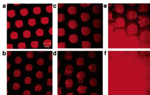
**Figure 3.** Confocal microscope images of dendrimers stamped using microcontact printing with circles of  $\sim 100 \mu\text{m}$  in diameter: (a) before immersion; (b) a uniform aldehyde substrate; (c–f) gradient substrates with increasing aldehyde concentrations, after 16 h of immersion in water.
