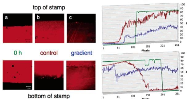
**Figure 2.** Confocal microscopy images of the top and bottom edges of stamped dendrimer regions (a) before immersion on a uniform aldehyde substrate, (b) after 16 h immersion in water, and (c) after 16 h immersion on a 15 min gradient substrate. The graphs on the right show the averaged fluorescence intensity profile<sup>11</sup> of each picture from top to bottom ((a) green, (b) red, (c) blue).
